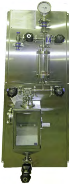
Free standing vessel sampling system for sampling unstable process liquor with self-draining, zero crevice design, and eductor to generate vacuum.
