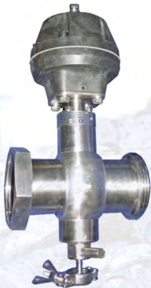
Actuated In-Line sample valve with DIN11851 end connections & triclamp sample outlet with purge connection.
