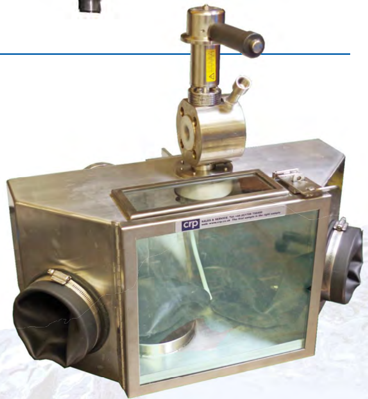
Cabinet with glove ports and padlockable latch
